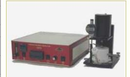
TBS 2100*E-F* Viscometer can be operated in *Manual* mode as shown above. Automation systems can be easily integrated later.
