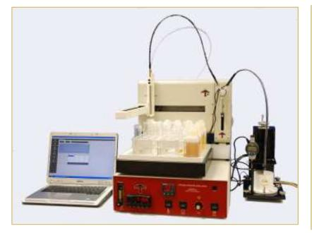
There are two TBS automation packages available -- one with a multi-position AutoSampler and one without. Both packages incorporate a Laptop for automated rotor/stator adjustments and instrument calibrations.
